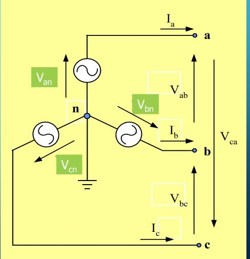
PHASE VOLTAGES,  $V_{\phi}$
