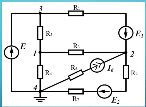
If there is a branch between two nodes containing an ideal EMF and does not contain passive elements, then when grounding one of these nodes (for example, node 4), to wit assuming  $\varphi 4 = 0$ , it is easy to find the potential of node 3, since  $\varphi 3 - \varphi 4 = E$ , and from it  $\varphi 3 = E$ .
