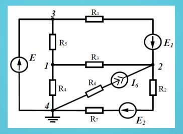
When finding own and joint conductances in this system, it should be taken into account that branch 6 contains an ideal current source. As indicated earlier, the current in this circuit is equal to the current of the current source I6, and the internal resistance of the ideal current source is infinitely large, so the conductivity of this circuit Y6 = 0.
