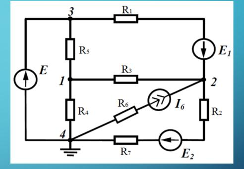
$I_{11} = 0,$  $I_{22} = E_1 \frac{1}{R_1} - E_2 \frac{1}{R_2 + R_7} + I_6.$
