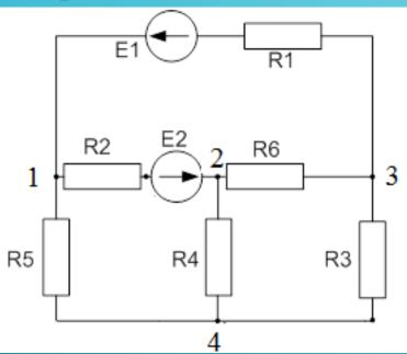
Ground node 4 and write down the system of equations using the nodal potential method in general form:
