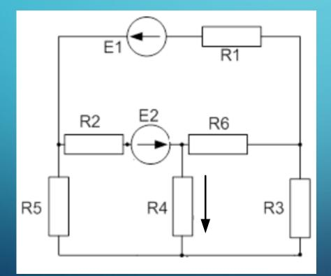
R1 = 15 Ohm R2 = 20 Ohm R3 = 10 Ohm R4 = 25 Ohm R5 = 25 Ohm R5 = 25 Ohm R6 = 15 Ohm E1 = 150 V E2 = 120 V
