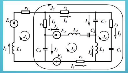
There are four independent loops in the circle. Let's set the direction of the loop currents as shown in the figure, and write the equation for four loops in general form:
