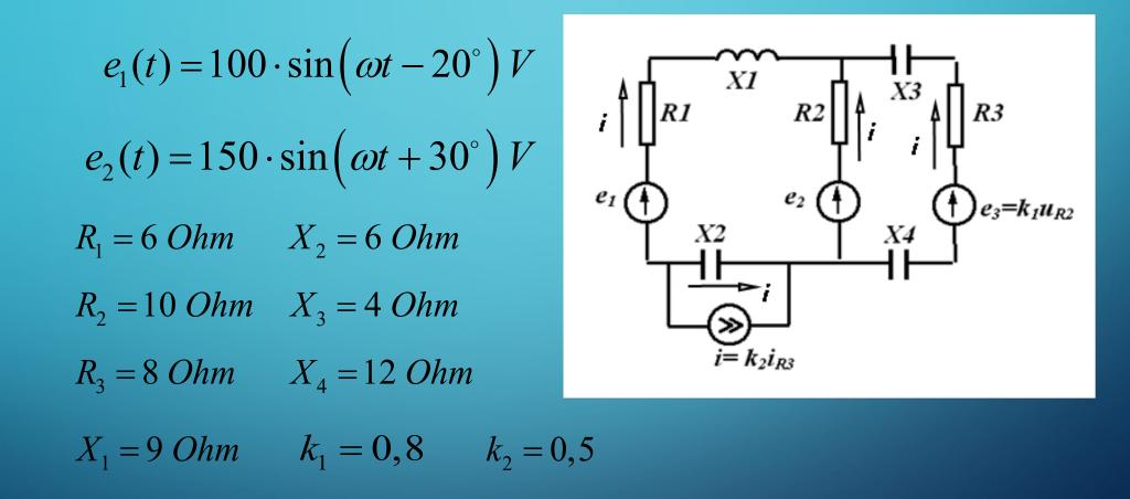
Let's write the expressions for the complete complex resistances of the circuits, assuming that the circuit number coincides with the current number
