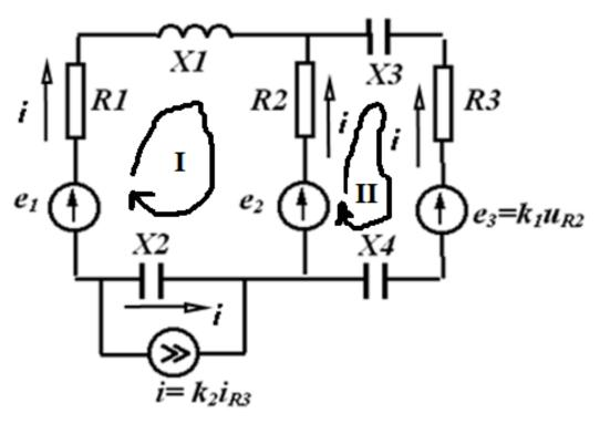
$\underline{E}_3 = k_1 \underline{I}_2 \underline{Z}_2 \qquad \underline{I} = k_2 \underline{I}_3$
