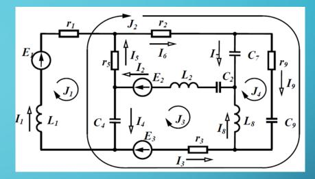
$\underline{Z}_{23} = \underline{Z}_{32} = r_3 - j \frac{1}{\omega C_{\star}},$
