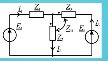
Let's formulate the rules for compiling equations according to Kirchhoff's laws for circles with mutual inductive connections. Consider this on the example of a two-circuit circuit (figure). We arbitrarily specify the directions of the branch currents. Uncoordinated switching of the coils corresponds to these directions.
