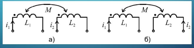
The symbols (•), ( $\Delta$ ), (\*) on the electrical diagrams indicate the conditional beginnings of the coil. If the currents are oriented in the same way relative to such  $\mathcal{P}$  markings, then the inclusion is consistent.
