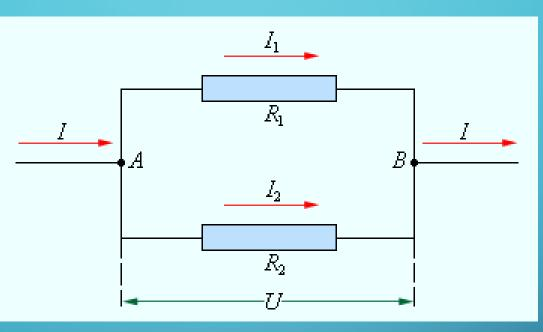
When connected in parallel, the current is greater in the conductor with lower resistance.
