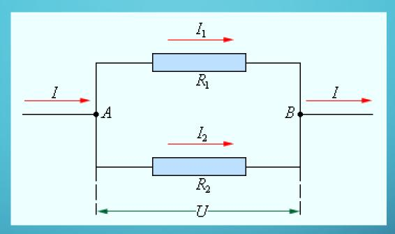
• The voltage at the ends of conductors connected in parallel is the same:
