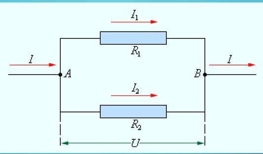
• Applying Ohm's rule for a section of a circle, it can be proved that
