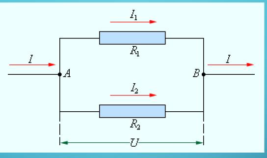
• Since electric charge does not accumulate at the branching point, the charge arriving at the node per unit of time is equal to the charge leaving the node during the same time. So:
