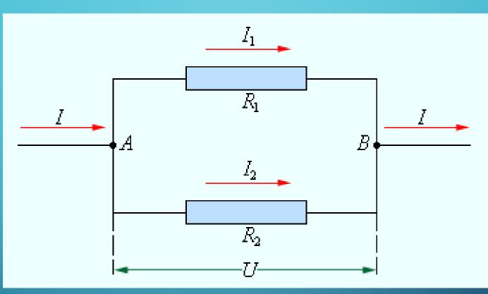
• With a parallel connection, the ends of the elements of the electric circuit are connected.
