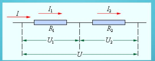
The strength of the current in all conductors is the same, since the electric charge does not accumulate in them and the same charge passes through any cross-section of the conductor in a certain time
