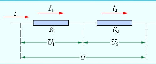
• The voltage at the ends of this section of the circle consists of the voltages on each conductor:
