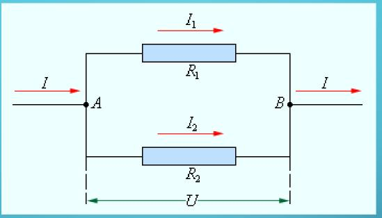
With a parallel connection, the current in the section of the circuit is inversely proportional to its resistance:
