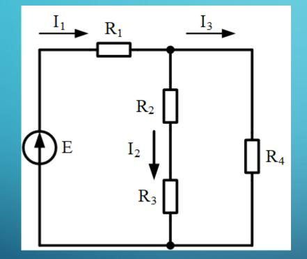
$R_5 = R_2 + R_3$
