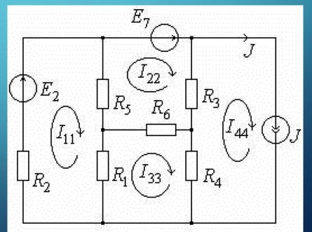
The circle has four independent loops. According to the method of loop currents, three equations need to be compiled, since the loop current  $I_{44}$ =J is known. Let's write the system of equations according to the method of loop currents in general form:
