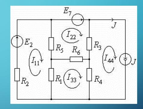
Own EMF:  $E_{11} = E_2 = 20 \ (V),$   $E_{22} = E_7 = 24 \ (V),$  $E_{33} = 0 \ (V).$  Let's substitute the values into the system of equations:
