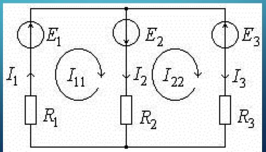
According to Kirchhoff's second rule:  $E_2$  $I_1 R_1 + I_2 R_2 = E_1 + E_2,$  $I_1$  $-I_2R_2 + I_3R_3 = -E_2 - E_3.$  $R_1$ Express the currents in the branches in terms of loop currents:  $I_{11}R_1 + (I_{11} - I_{22})R_2 = E_1 + E_2,$  $-(I_{11}-I_{22})R_2+I_{22}R_3=-E_2-E_3,$ or  $I_{11}(R_1+R_2)-I_{22}R_2=E_1+E_2,$  $-I_{11}R_2 + I_{22}(R_2 + R_3) = -E_2 - E_3.$
