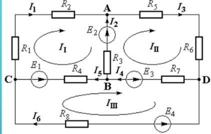
Let's select three independent loops in the circle and write the system of equations according to the method of loop currents in the general form:
