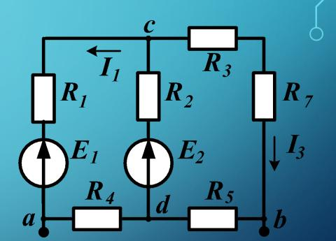
$\boldsymbol{\varphi}_a = \boldsymbol{\varphi}_d + \boldsymbol{I}_1 \boldsymbol{R}_4 \qquad \boldsymbol{\varphi}_b = \boldsymbol{\varphi}_d + \boldsymbol{I}_3 \boldsymbol{R}_5$
