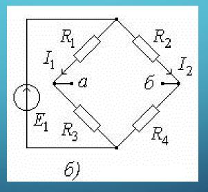
$U_{a\delta} = E_e = -I_1R_1 + I_2R_2 = -\frac{E_1R_1}{R_1 + R_3} + \frac{E_1R_2}{R_2 + R_4} = \frac{E_1(R_2(R_1 + R_3) - R_1(R_2 + R_4))}{(R_1 + R_3)(R_2 + R_4)}$
