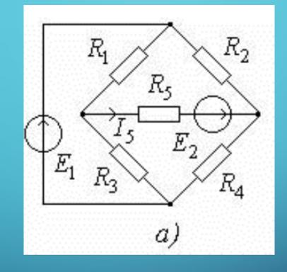
$$I_{5} = \frac{U_{a\delta} + E_{2}}{R_{ex} + R_{5}} = \frac{E_{e} + E_{2}}{R_{e} + R_{5}}.$$
