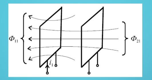
If the magnetic flux coupled to a given circuit is formed by the current of another circuit, then such a flux is called a mutual induction flux, and the corresponding flux linkage is a mutual induction flux linkage.
