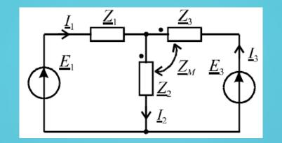
Let's formulate the rules for compiling equations according to Kirchhoff's laws for circles with mutual inductive connections. Consider this on the example of a two-circuit circuit (figure). We arbitrarily specify the directions of the branch currents. Uncoordinated switching of the coils corresponds to these directions.
