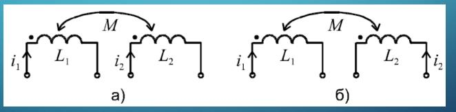
The symbols  $(\bullet)$ ,  $(\Delta)$ , (\*) on the electrical diagrams indicate the conditional beginnings of the coil. If the currents are oriented in the same way relative to such  $\mathcal{P}$  markings, then the inclusion is consistent.
