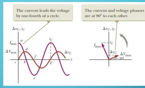
Instantaneous current and voltage are out of phase by  $\pi/2$
