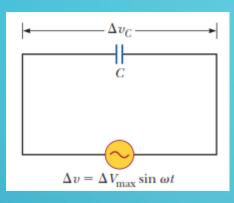
$\Delta v + \Delta v_C = 0$  $\Delta v - \frac{q}{C} = 0$  $q = C\Delta V_{\text{max}} \sin \omega t$  $i = \frac{dq}{dq} = \omega C\Delta V$
