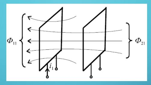
The magnetic flux  $\Phi$  in loop, which is formed by the electric current I of this loop, is called the magnetic flux of self-induction (figure). Corresponding to this, the flux linkage of the loop (coils)
