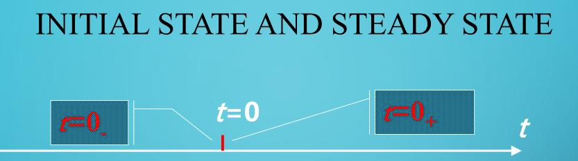
Assume changing circuit when t=0, then t=0- is end point of old steady state; t=0+ is the start point of transient state.
