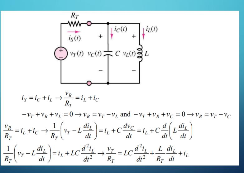
$$a_2 \frac{d^2 x(t)}{dt^2} + a_1 \frac{dx(t)}{dt} + a_0 x(t) = b_0 f(t) \rightarrow \frac{1}{\omega_n^2} \frac{d^2 x(t)}{dt^2} + \frac{2\zeta}{\omega_n} \frac{dx(t)}{dt} + x(t) = K_S f(t)$$
