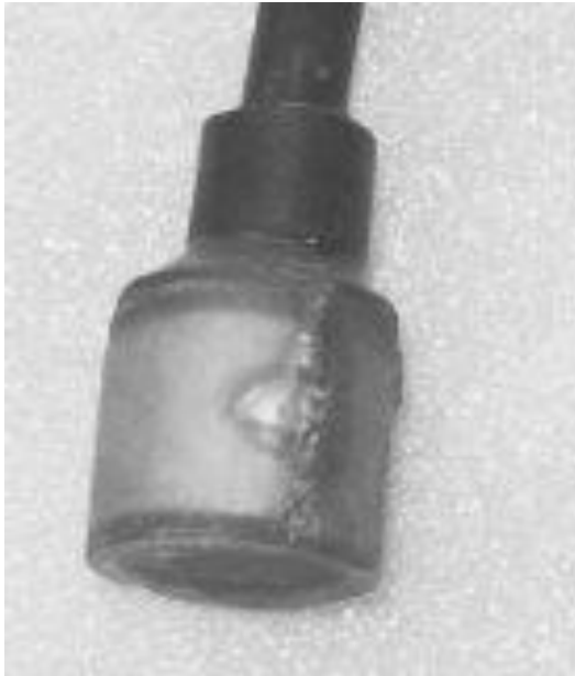
Fig. 1. Measuring hydrophone based on piezoceramic
