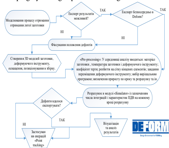
Fig. 4. Algorithm for the simulation of through technological processes in software complexes of finite-element modeling of the DEFORM-3D type
