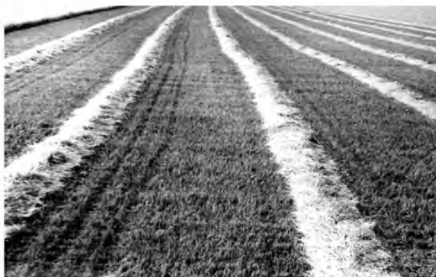
Fig. 6. View of swaths formed by swath reaper at speed of working movement of harvesting machine-and-tractor aggregate equal to 3.8 \text{ m}\cdot\text{s}^{-1}
