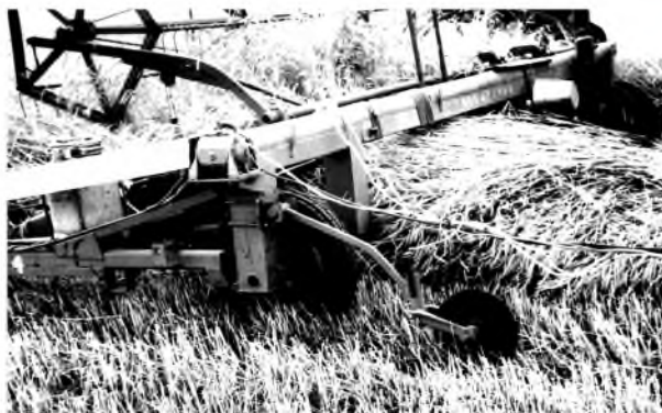
Fig. 2. Track-measuring wheel, installed on trailed swath reaper
