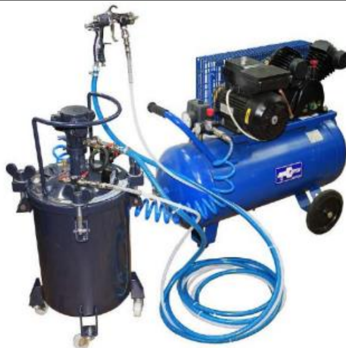
Figure 6 - Paint injection tank with spray gun and compressor.
