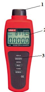
Figure 4. UNI-T UT372 frequency meter: 1 – laser reader; 2 – digital indicator; 3 – control panel
