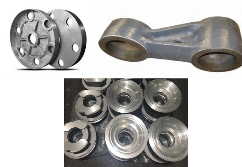
Fig. 1. Samples made by isothermal stamping
