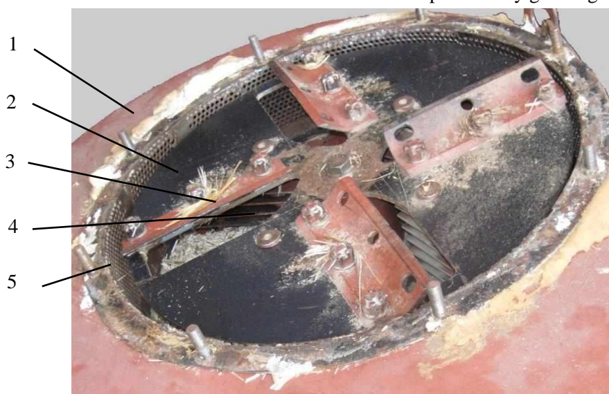
Fig. 1. Hammer grinder of plant raw materials (with the loading neck removed): 1 – body; 2 – disk with slots; 3 – pre-grinding knife; 4 – package of hammers; 5 – sieve
