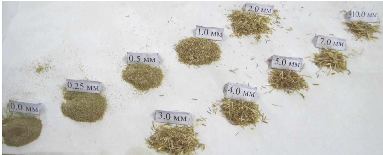
Fig. 3. Samples of fractions of crushed wheat straw obtained on sieves with appropriate holes
