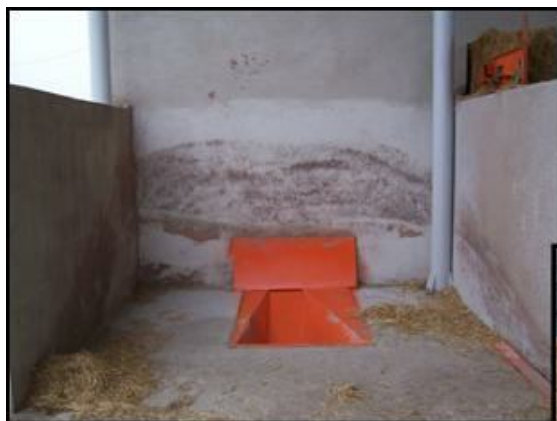
Picture 5 The waste after grain cleaning dosing on the post-harvest line
